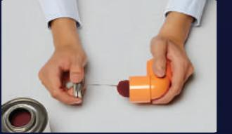
6 Apply CPVC Solvent Cement to the inside surface of the fitting 2-3 times. Repeat Step 5
